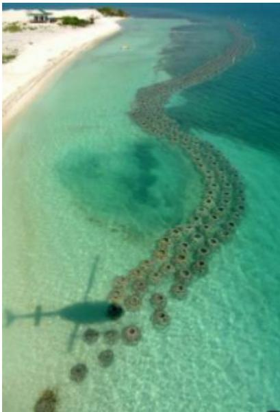
Top view breakwater from reef balls
